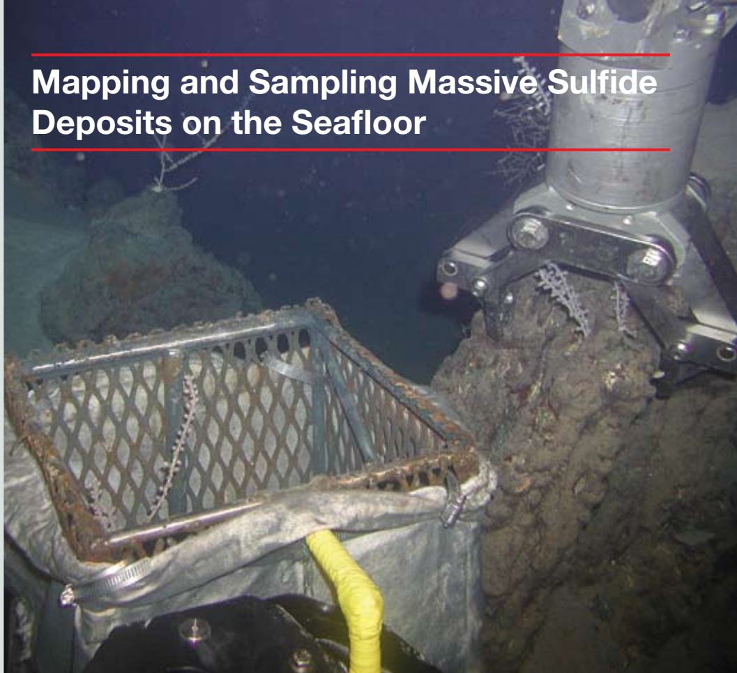
Remote Operated Vehicle (ROV) grab sampling at a water depth of more than 1600m
