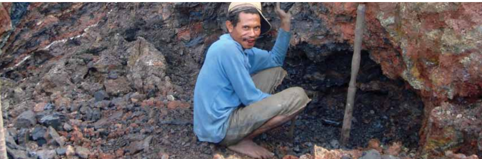
Typical bedded manganese deposit and artisanal extraction techniques, West Timor (above); Massive chert manganese breccia deposits, unconformity related, with local owners, West Timor (left)
