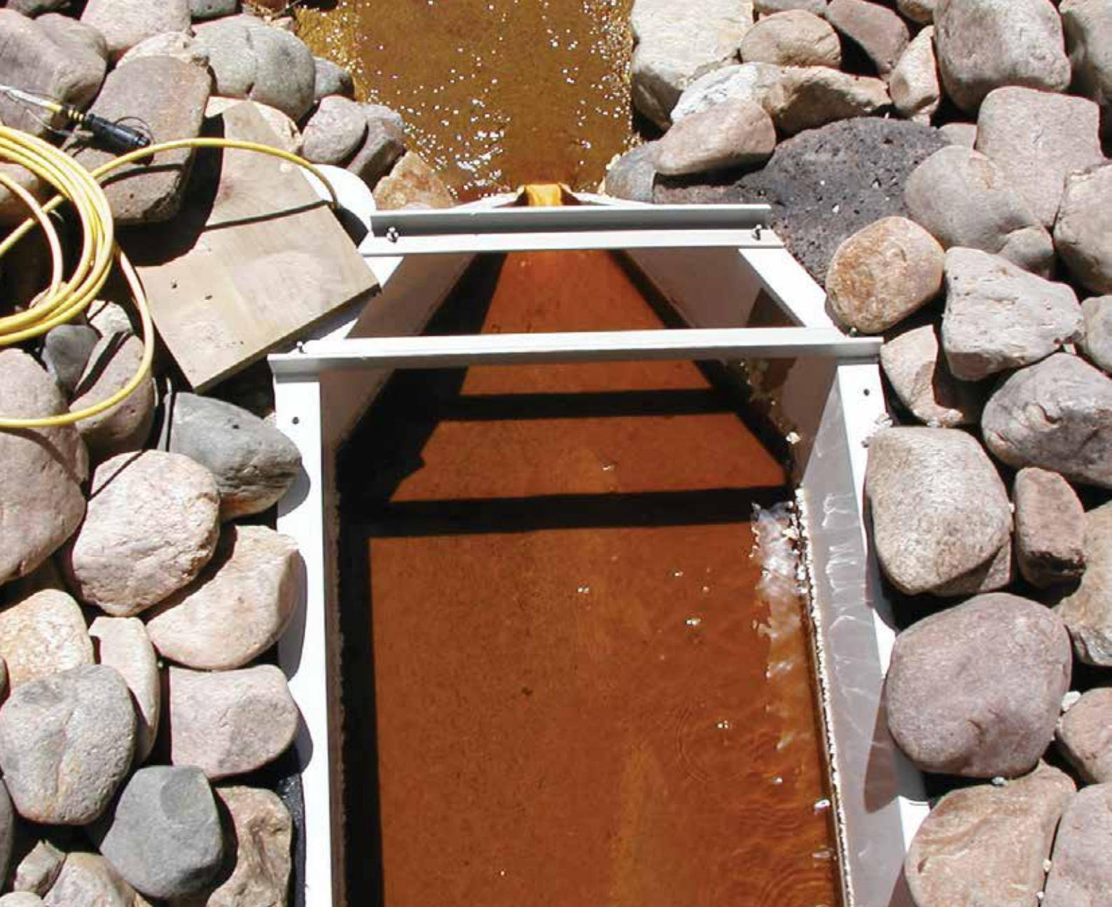
Continuous flow measurement of seepage from rock pile, Questa Mine, New Mexico
