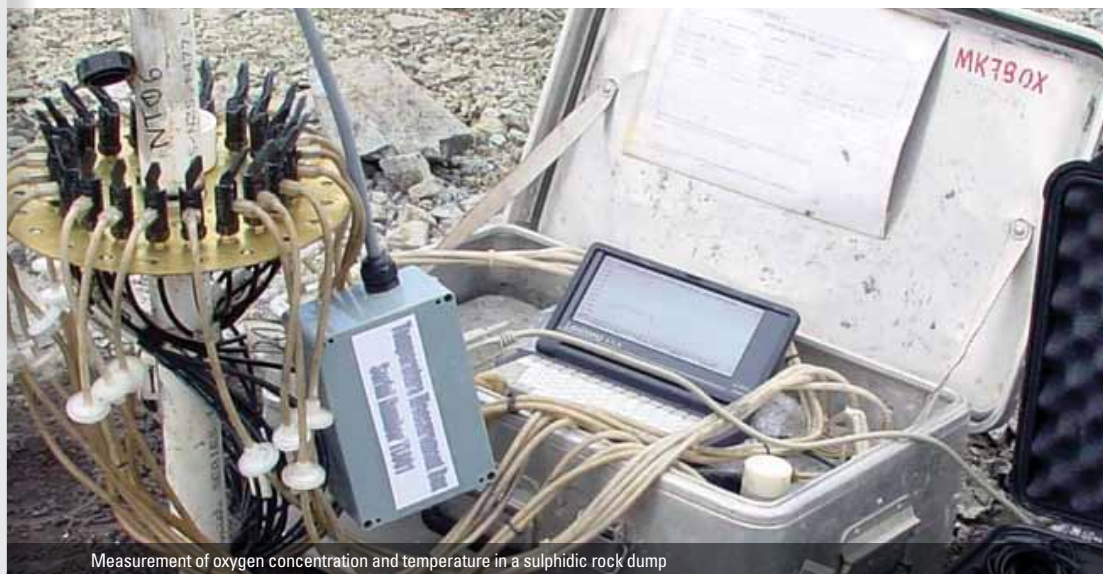
Measurement of oxygen concentration and temperature in a sulphidic rock dump
