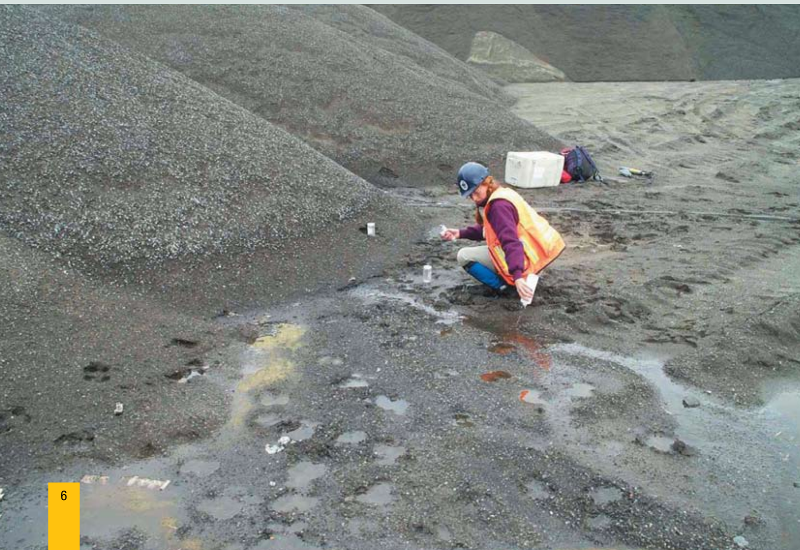
SRK's Kelly Sexsmith sampling seepage from coarse kimberlite rejects at the Ekati Diamond Mine™
