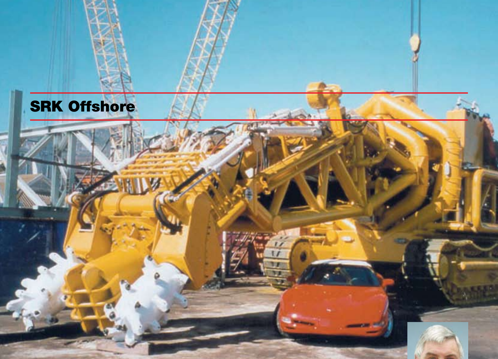
Undersea mining unit used to extract sediments from the sea floor
