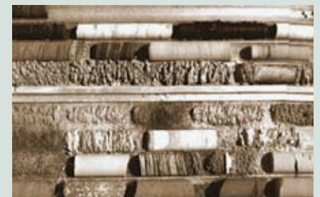
The kimberlite core samples above are shown below after only 3 wetting and drying cycles – many with extensive deterioration
