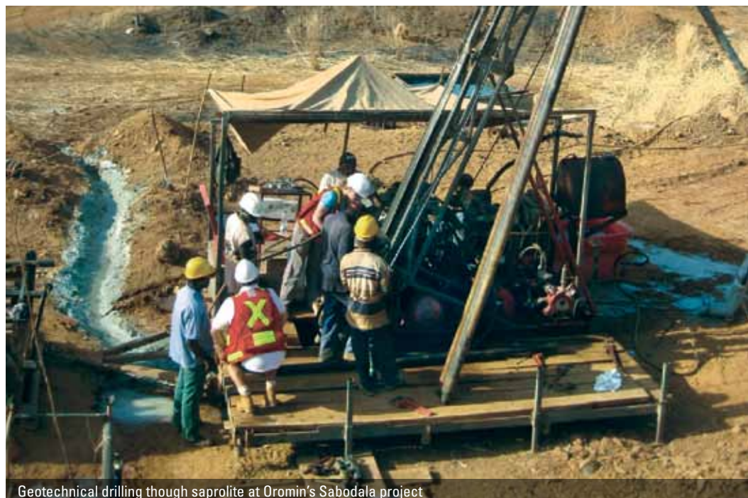
Geotechnical drilling through saprolite at Oromin's Sabodala project
