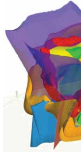
Leapfrog Geo, 3D model of surface geological interpretation based on surface mapping and structural data (left) 3D model section through an overturned Stratiform Base Metal Sulphide model and fault network produced in Leapfrog Geo (right)
