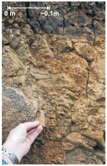
Figure 5: Highly plastic clay with nuggety fractured structure.
