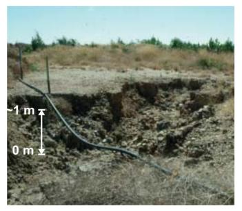
*Figure 7: Erosional gully in fine-grained soil due to high intensity storm.*
