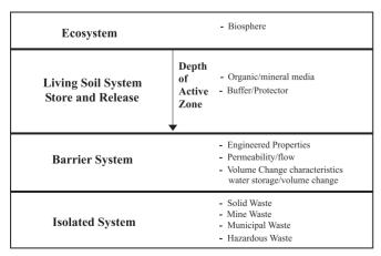
Figure 2: Appropriate concepts for the design of a soil cover system.
