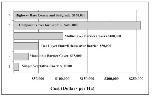
*Figure 8: Indicative costs for cover construction. Dollar amounts are approximate for construction in Australia, Canada and the United States, in local currency.*
