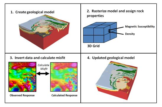
Figure 3: Generalised workflow of the constrained inversion process
