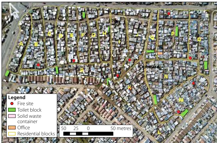
Figure 4 Following testing done at Stellenbosch University, thousands of smoke alarms have now been rolled out across the Western Cape in informal settlements. The figure shows where activations occurred in the Wallacedene TRA settlement after the installation of a smoke detector in every dwelling [8]
