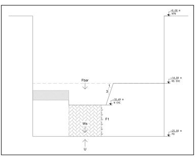
Figure 12. Forces acting on the soil plug in region 1-B.
