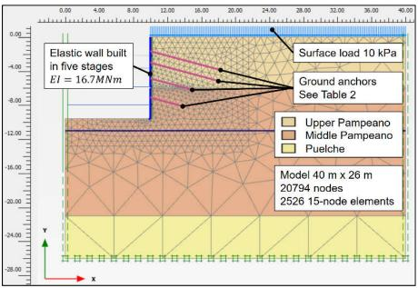
Figure 16. Geometry and finite element mesh.
