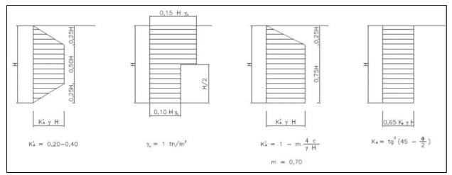
Figure 4. Code diagrams of minimum design earth pressures for strutted excavations i) Stiff clays; ii) Pampeano Fm.; iii) Soft clays; iv) Sands (Moretto 1972).
