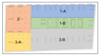
Figure 11. Division of the excavation area to prevent bottom uplift failure.
