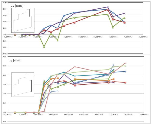
Figure 8. Horizontal displacements of selected control points at the crest of the wall.
