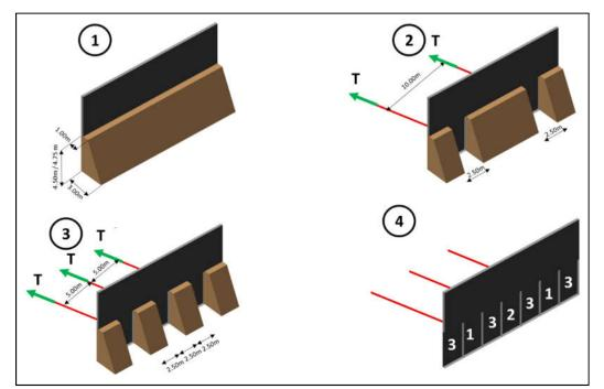
Figure 5. Typical construction procedures for large excavations in Buenos Aires. Ideal sketch.
