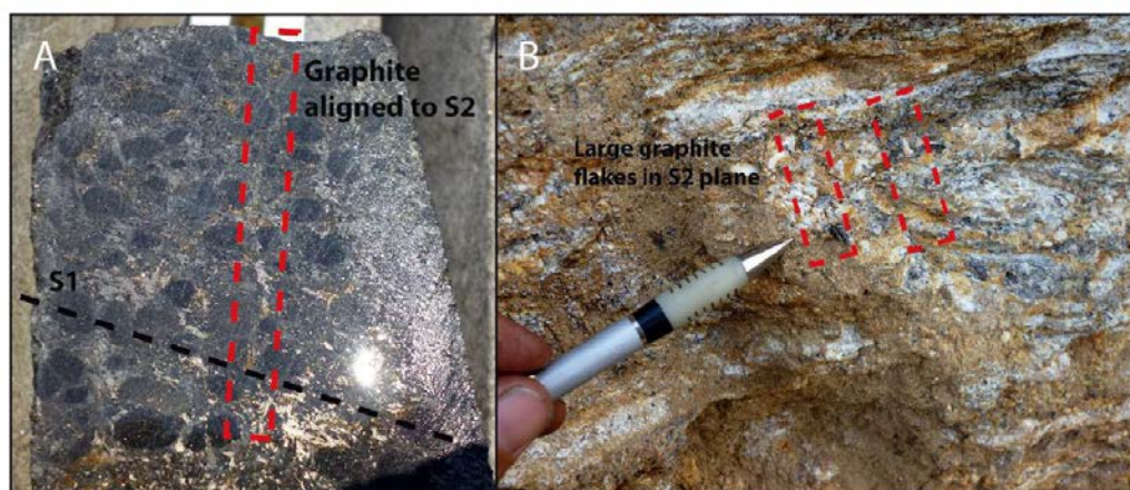
Figure 2: Structural control of graphite mineralisation in the Epanko Project; A – Graphite aligned to the S 1 and S 2 fabrics within drill core; B – Large graphite flakes forming along the S 2 plane
