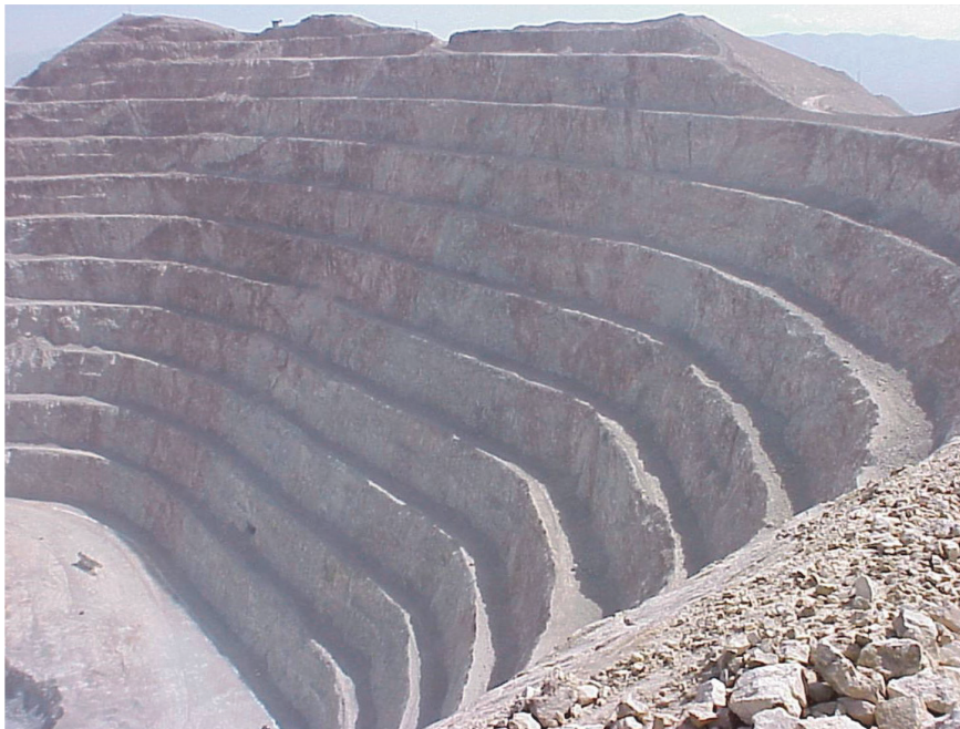
Figure 7. View of a benched slope in an open pit mine used to illustrate the application of the proposed stability analysis tools.
