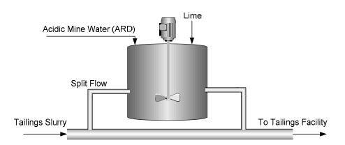
Figure 5 - Schematic of potential implementation of in-plant ARD treatment
