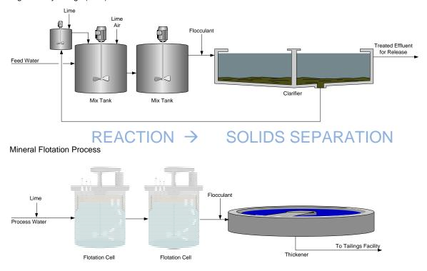
High Density Sludge (HDS) Water Treatment Process
