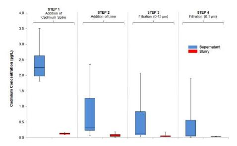
Figure 2 - Bench-scale test results for cadmium removal from tailing slurry and tailings supernatant
