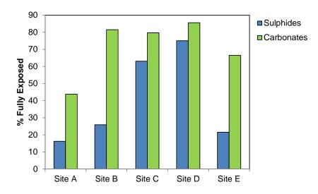
Figure 6 – Comparison of sulphide and carbonate mineral exposure for tailings site samples
