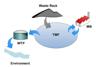
Figure 3 – Typical mine water management scenario
