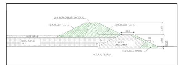
Figure 6. Typical cross section of a evaporation pond-salt stack for a project in the lithium triangle – internal database, SRK.
