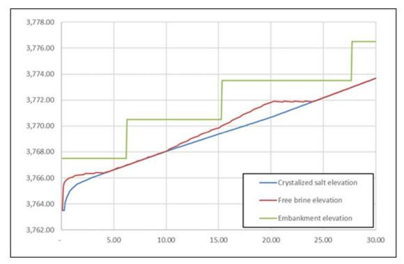
Figure 5. Brine storage level, crystallized salt elevation and embankment raising evolution over time for a project in the lithium triangle – internal database, SRK.
