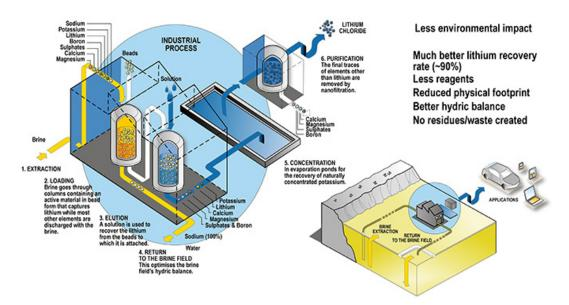
Direct Extraction Process is simple, efficient, low-cost and more environmentally friendly than conventional evaporation process
