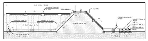
Figure 7. Typical cross-section of the starter embankment on the disposal spine side of a facility.
