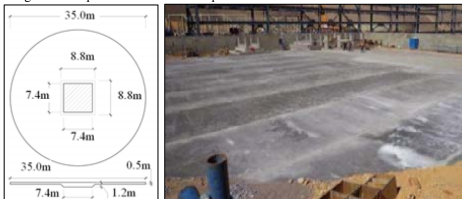
Figure 2-2. Circular stall sketch with central reinforcement (left) and casted on-site stall (right).
