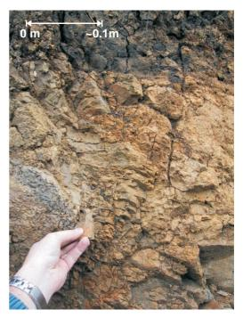
FIG 5 - Highly plastic clay with nuggety fractured structure.
