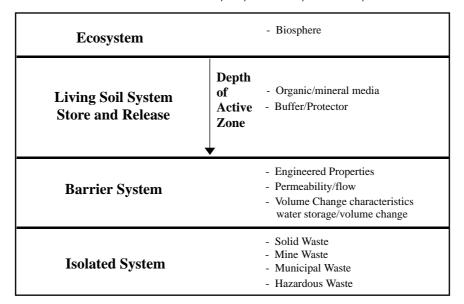
FIG 2 - Appropriate concepts for the design of a soil cover system.
