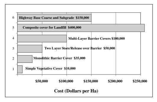
FIG 8 - Indicative costs for cover construction. Dollar amounts are approximate for construction in Australia, Canada and the United States, in local currency.
