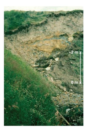
FIG 6 - View of erosional slump failure in an over-steepened slope.
