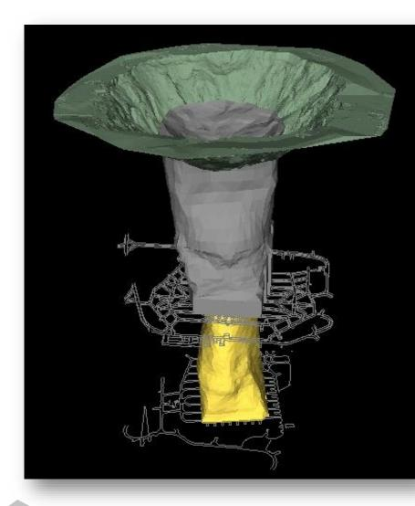
The risk of poor subsidence estimates is typically related to infrastructure location outside the subsidence limits (below). In smaller footprints and strong rock masses the subsidence angles could be negative (overhang) resulting in ore loss and early dilution!
