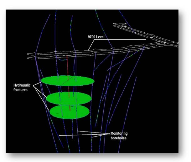
Transform a highly competent rock mass (primary rock) into a rock mass material appropriate for caving methods.
