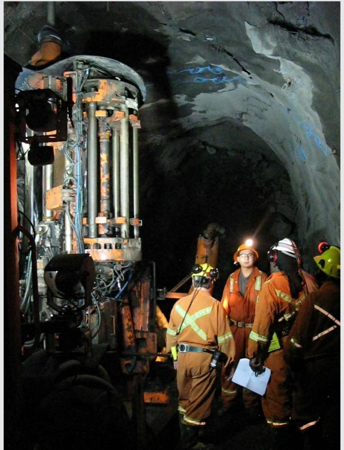
Figure 8: Solo production drill at Koala Mine.
