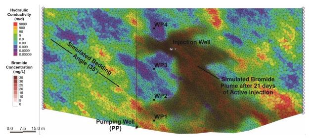
**Figure 1** Two-dimensional groundwater flow setup in FEFLOW. Simulated bromide plume and random K field are presented for the highest probability model generated using the external conditioning approach.
