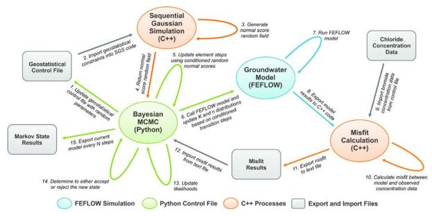
Figure 2 Overview of model structure using external conditioning approach.
