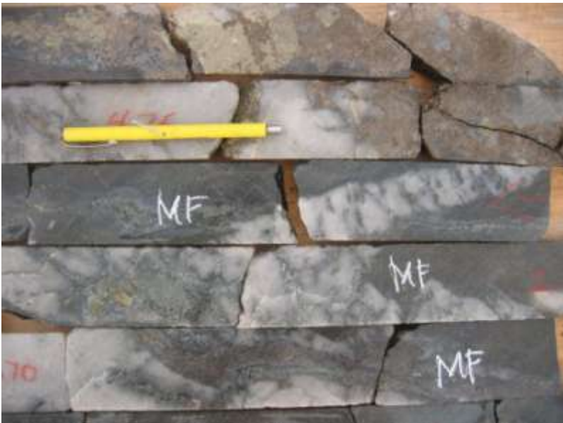
Quartz-carbonate and sulphide veins, Detour Lake
