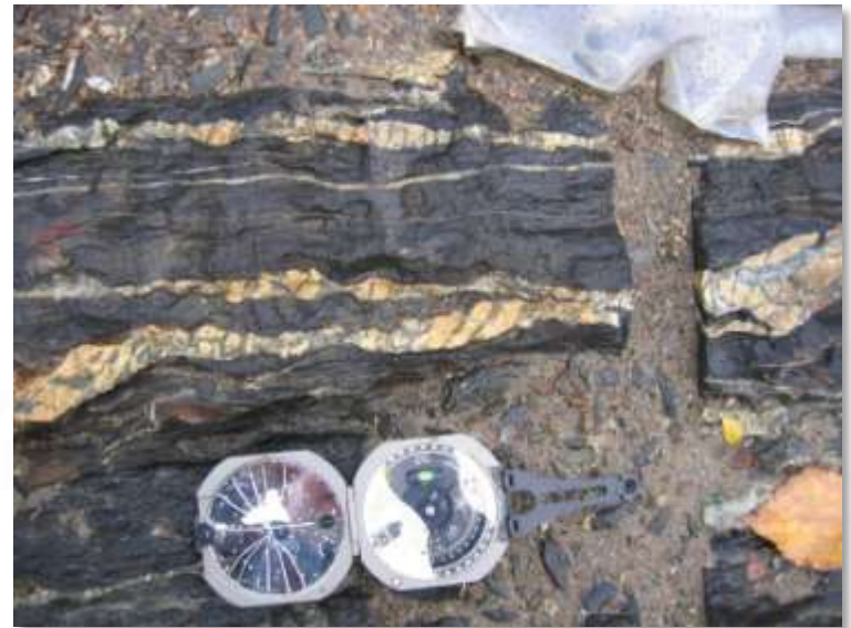
Quartz-amphibole vein infilling boudin necks in ankerite vein, Red Lake
