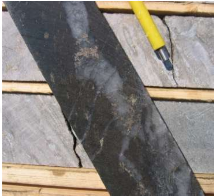
Pyrrhotite infilling a boudin neck in quartz vein
