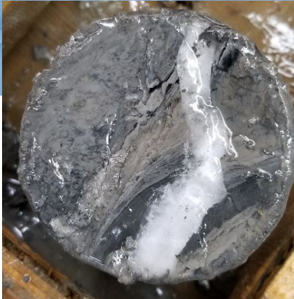
Ice-rich material present beneath the TIA
