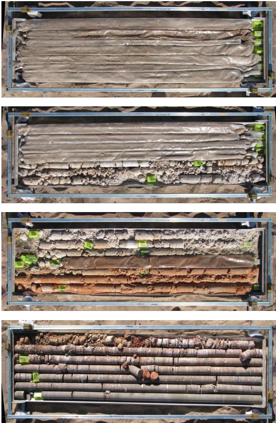
Figure 2: Borehole GT08-01 showing the Kalahari sequence, transitional and competent basalt
