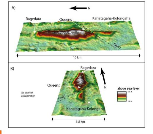
Topography showing double-plunging antiform and existing mines
