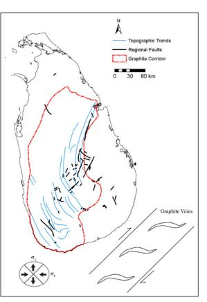
Associated with fold and re-folded double-plunging antiforms
