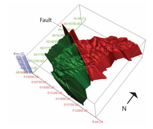
Modelled lodes offset and slightly rotated by NW-SE fault
