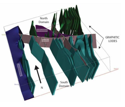
Modelled Graphitic Domains – North and South of fault
