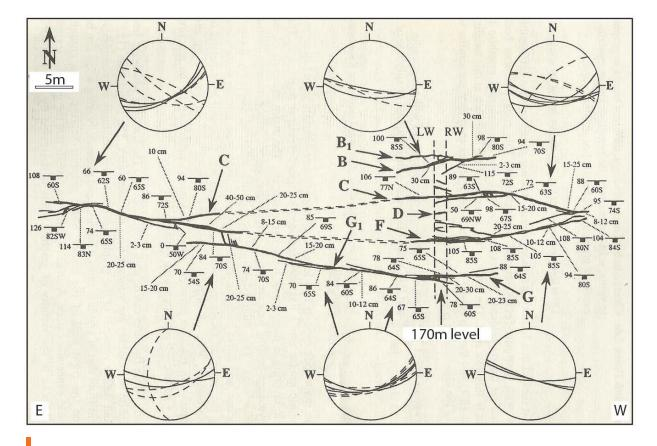
Sketch of graphite veins between 190 and 210m from main shaft at 170m RL
