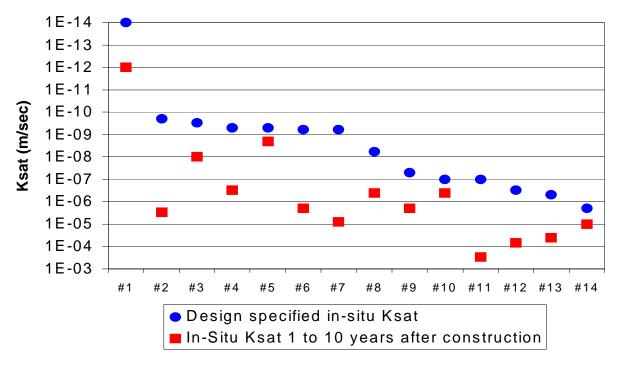
Figure 3. Case studies demonstrating how actual field measured hydraulic conductivities vary from those specified during the design stage.
