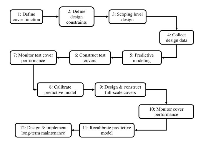
Figure 1. A proposed formalized cover design procedure as evaluated from the international cover design and construction review.
