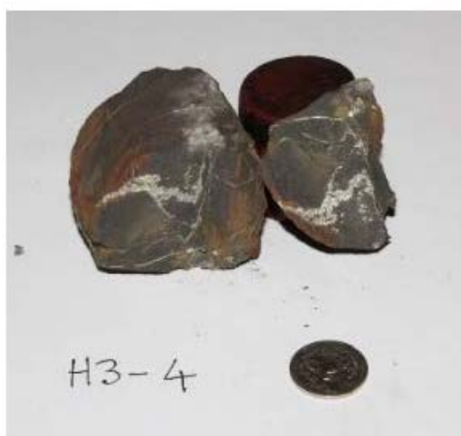
Figure 4: Photograph of siderite nodules containing marcasite/pyrite stringers
