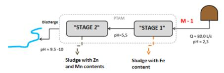
Figure 4. Typical scheme of the treatment system applying staged neutralization.
