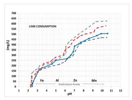
Figure 5. Neutralization curve and formation zones of Fe, Zn and Mn solid phases
