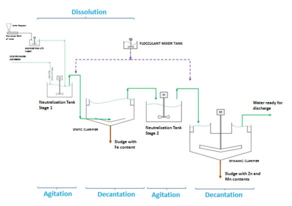
Figure 9. Unit operations in a staged treatment system.
