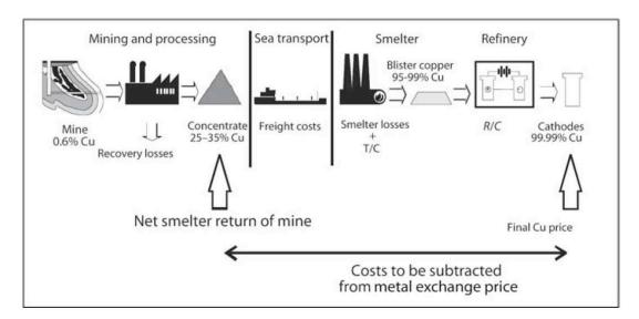
Figure 1: Schematic of NSR definition for a typical copper operation (Wellmer et al, 2008)
