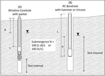
Figure 1: Airlift Submergence and Test Intervals for Tests in Coreholes and Air-Rotary Boreholes
