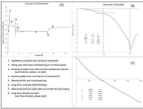
Figure 2: Hydrograph (A) and Hvorslev (C) and Theis (B) Analyses of a Typical Packer-Isolated Airlift-Recovery Test in a Deep Corehole.
