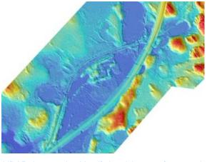
LiDAR data used to identify ice-rich permafrost terrain.
