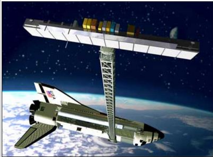
The SRTM antenna mast being deployed from Endeavour. Photo: DSS
