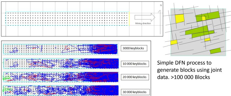
Limit equilibrium analysis – Monte-Carlo > 100 000 blocks Gravity fall, sliding, rotation – effect of support Keeps track of the surface area exposed for normalisation Unwedge image
