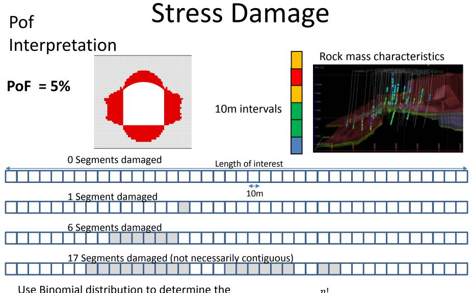
probability of various lengths of tunnel damage
